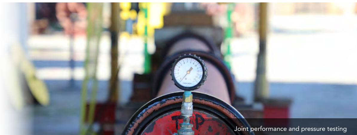
Compression joint test simulates joint performance under condition of shear and angular deflection
