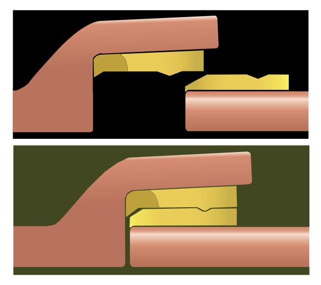
Shaded areas may be cast in some larger diameter joints, depending on manufacturing method.
