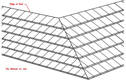
The detail to the left shows the field of roof tile completely laid. It is necessary to cut tiles on the job to fit the miter at all hips. The miter is filled with cement mortar and short pieces of miter tile are also bedded and held with cement mortar.
